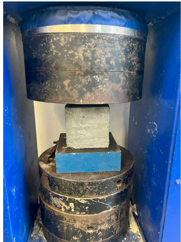
Concrete cube sample (10x10x10cm) undergoing compression strength test on the compression testing machine.
