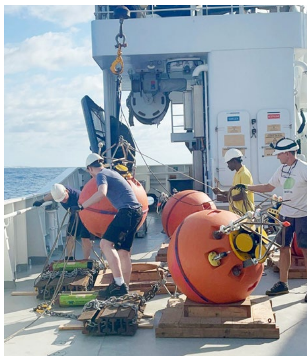
Moorings being prepared for deployment off Bazaruto (Mozambique) from the Norwegian research vessel Dr Fridtjof Nansen in 2023. These will measure ocean currents, temperatures, oxygen, salinity, and chlorophyll for nine months. The data will be used to validate an ocean model that Prof Mike Roberts' team is developing
