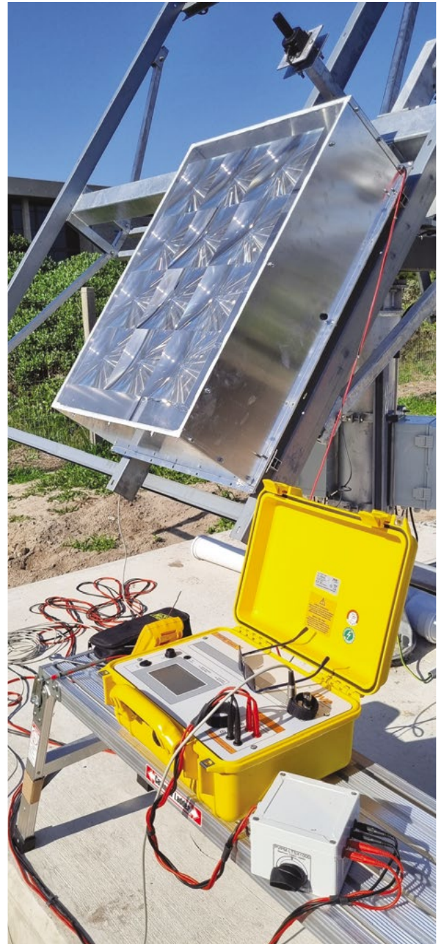
Patented Nelson Mandela University Hybrid CPV module undergoing testing
